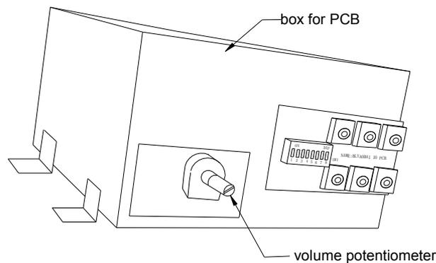
2. Turn the volume potentiometer to adjust the volume. Clockwisely turn the potentiometer to increase the volume; counterclockwisely will decrease the volume.
